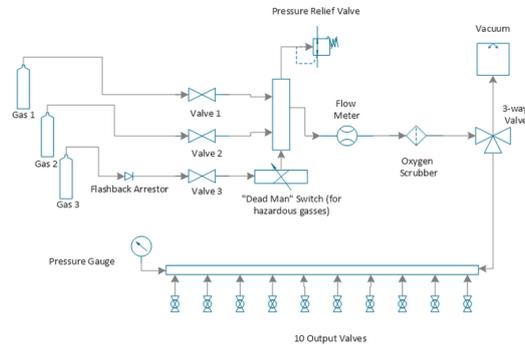
Figure 1: A simple drawing of the gas flow through the manifold
